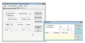
By making upper and lower limit settings it is possible to monitor measurements for warnings and when one occurs the unit's LED will flash. It is also possible to find out the time of the warning.
